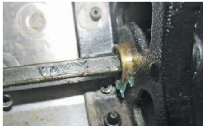
MSK07 kit adds an additional bushing for increased support and reduced freeplay.
