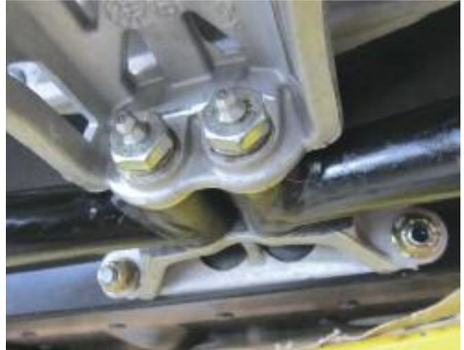
New lower A-arm bushing kit installed, ready for grease.
