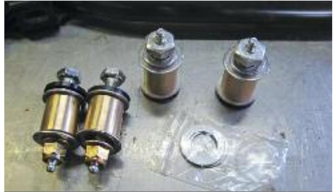
MSK02-1 Greasable Swing Arm Bushing Kit ready to install on the rear suspension's front arm.
