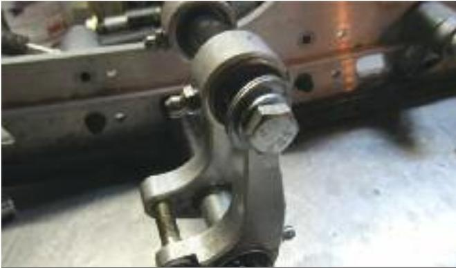
MSK03-1 Rocker Arm Bushing Kit adds new, wider bushings as well as grease fittings to both pivot points. This is the linkage between the centre and rear shock. Free movement is important
