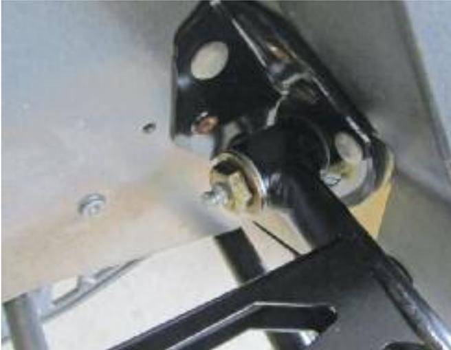
New upper A-arm bushing kit installed with easy access for the grease gun.
