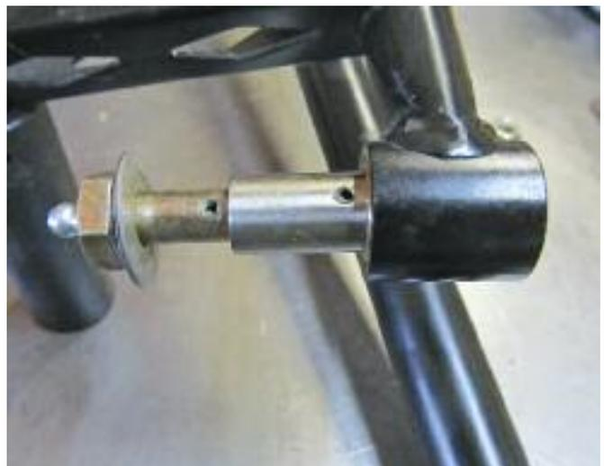
MSK01 Greasable Control Arm Kit. Note the ports for the grease to travel through the bolt to each pivot point.
