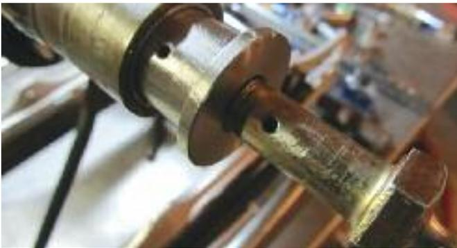
MSK05-1 SC-5 Rear Arm Bushing Kit. Note how easy it is to provide grease to this important pivot point."
